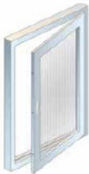
Hinged windows can open inward or outward.
