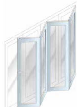
Bi-fold doors are hinged to fold neatly to one side in a concertina style.
